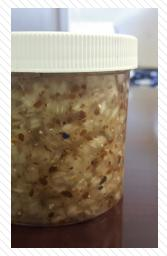
With a specific gravity of 1.17, Durafiber-X also does not float, nor does it sink, suspending itself evenly throughout a mixture.
